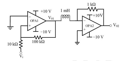
Assume that the initial inductor current is 0 A. The input voltage (V<sub>i</sub>) is a triangular signal with peak voltages of  $\pm 2$  V and time period of 8 µs. Which one of the following statements is true?
